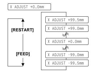
**[FEED]** key: Pressing the **[FEED]** key one time causes a -0.5mm :hange, up to -99.5 mm.
